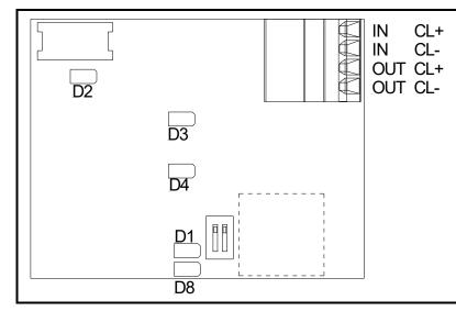
1: OFF default 2: OFF Terminal: Signal: IN CL+ Input Data + IN CL-Input Data -OUT CL+ Output Data +
